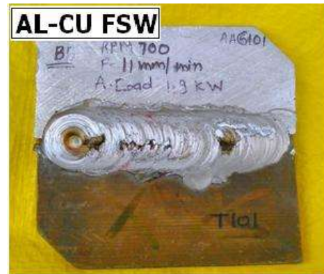
Photograph of Dissimilar joint Copper and Aluminium AA6101
